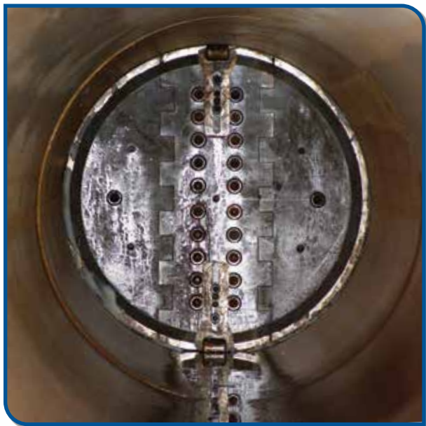
24" x 16" LINE STOP FOLDING HEAD
