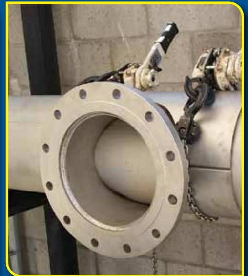
12" x 12" SS WELD-ON NOZZLE W/WRAPPER PADS
